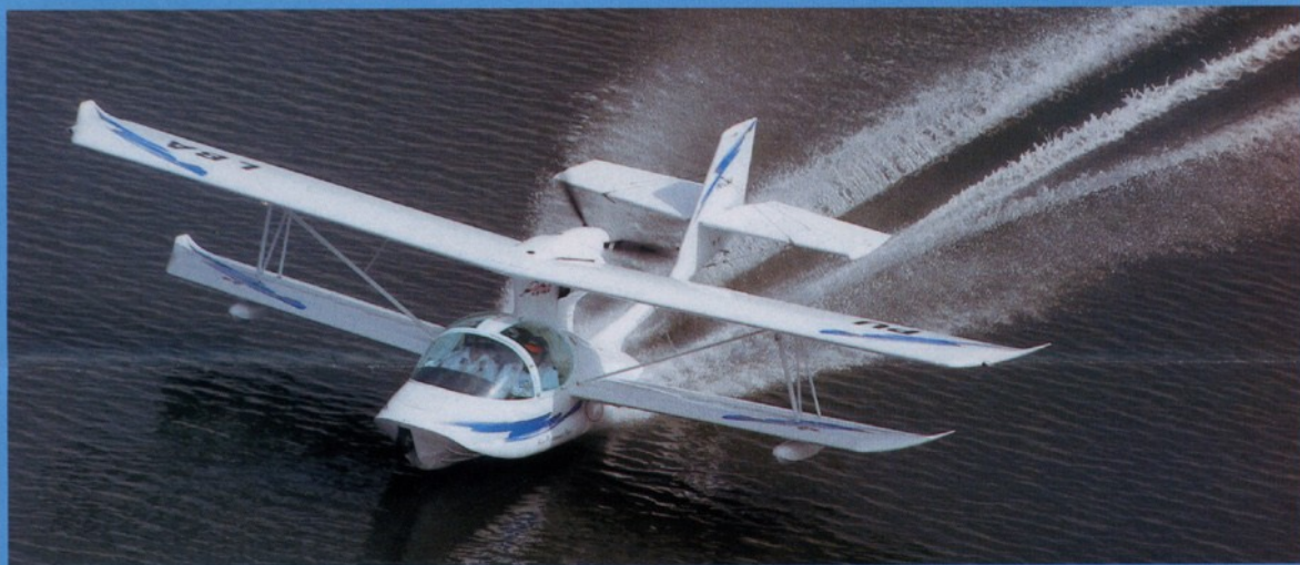
The tailplane and rudder are wire-braced.
