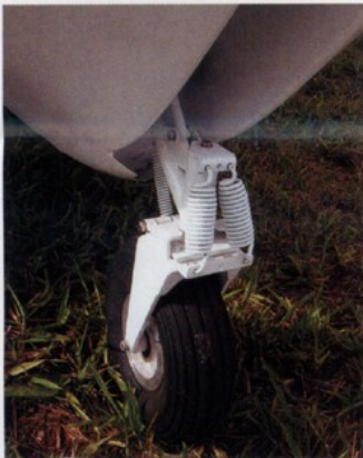
LEFT The nose wheel is carried by a leg made of 4130 chromoly steel, while the fork is 6061-T6 aluminium. Springs absorb the landing loads.
